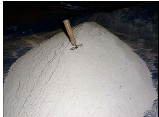
Plate 6 APC after coning
