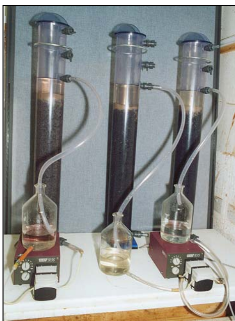
Plate 11 Columns filled with bottom ash
