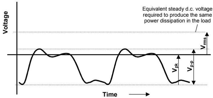
Figure A2.4 An alternative periodic waveform illustrating the magnitude of  $V_{pk}$ ,  $V_{p-p}$ ,  $V_{rms}$ .
