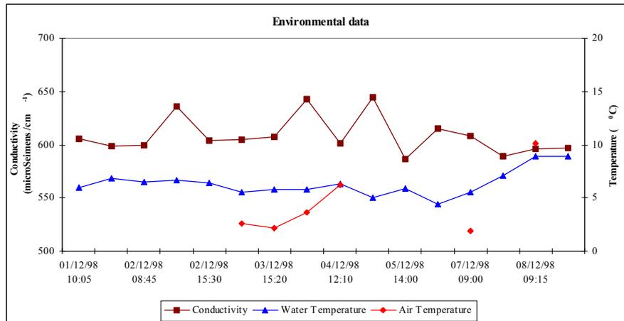
**Figure 6.4:** Water conductivity (corrected to 25°C), water temperature and air temperature readings recorded during the WAVE experiment
