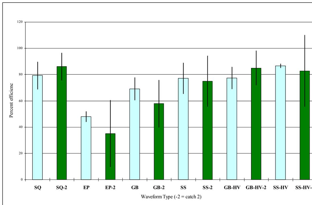
Figure 6.5 Mean (+/- 95% CL) catch efficiencies for different waveforms (-2 = second catch)
