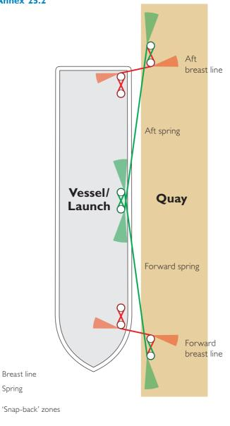
The full and safe Mooring Arrangement for small **Domestic, Passenger Craft and Ships Launches** illustrating potential 'Snap-Back' Zones
