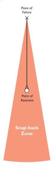
Diagram I - A Simple Mooring System Illustrating The Potential "Snap-Back" Zone Area
