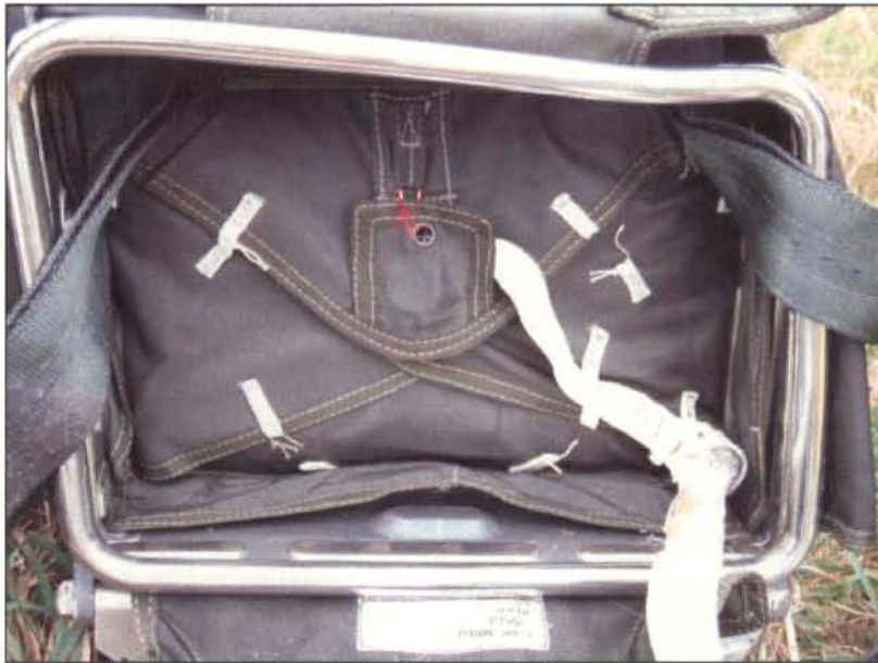
Figure 35 – XX177 Duplex Drogue and Parachute Container.
