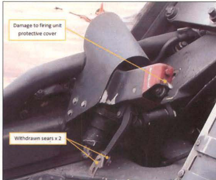
Figure 33 – XX177 Front Cockpit MDC firing unit and lever.
