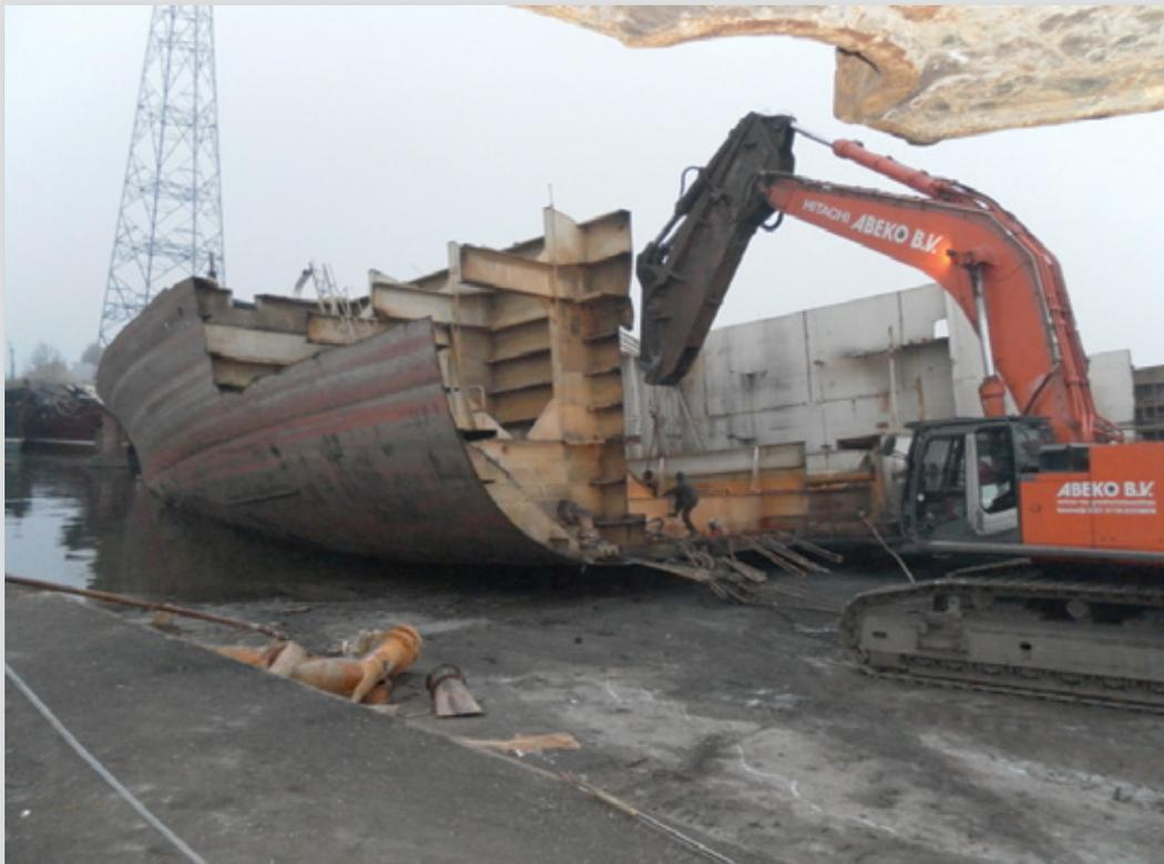
Final stages of dismantling with just the engine room left
