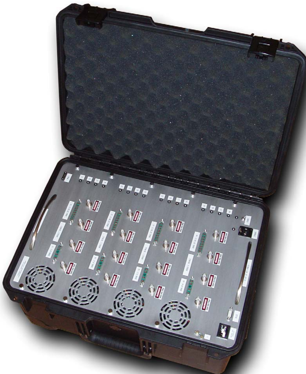
The 16-channel Pulse Shape Discriminator Module
