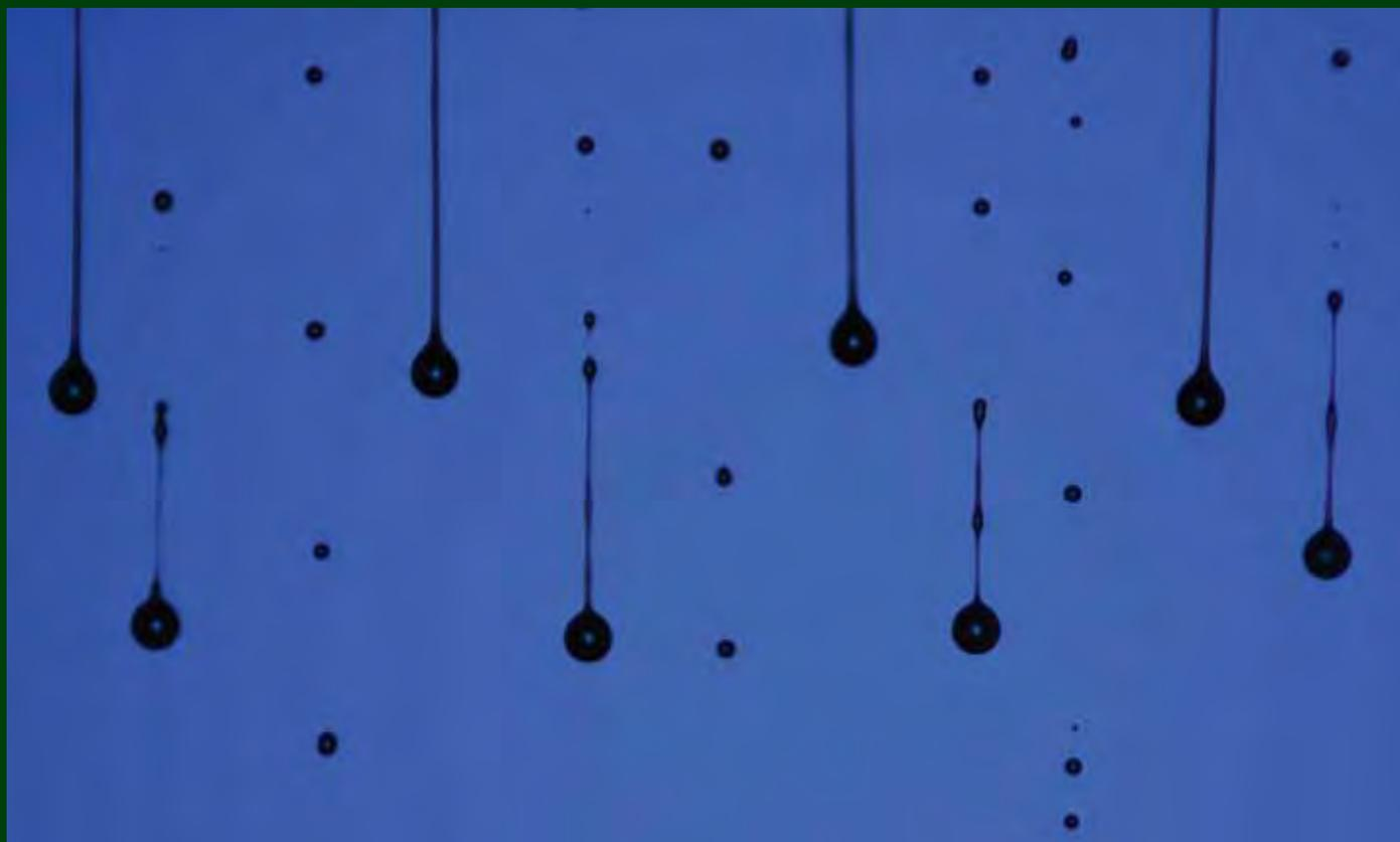
**Above:** This image captured with a very brief (20 ns) flash shows jets of ink ejected from an array of 11 nozzles at the top of the frame. Credit: University of Cambridge, Inkjet Research Centre.
