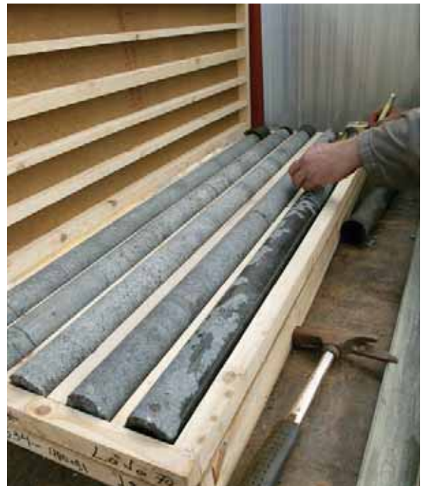
Measurements of drill cores from test drilling in Sweden (courtesy SKB)
