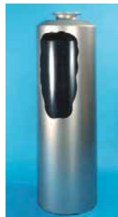
Cutaway showing simulated vitrified HLW in a stainless steel container (courtesy BNFL)
