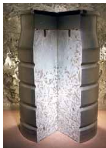
Cutaway showing simulated conditioned ILW in a stainless steel container (courtesy BNFL)
