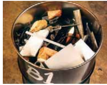
Drum of raw LLW of miscellaneous materials (courtesy BNFL)
