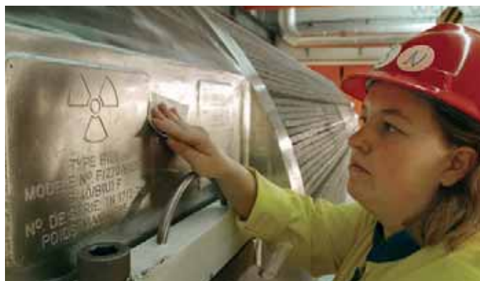
Transport cask in the reception area of Swedish central interim storage facility for spent nuclear fuel (courtesy SKB)
