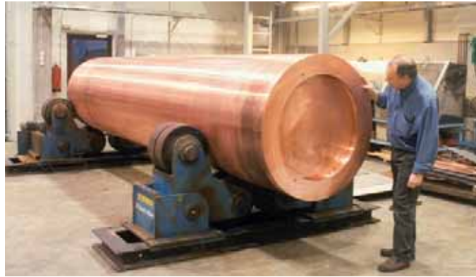
Copper cylinder for spent fuel disposal in Finland (courtesy Posiva)
