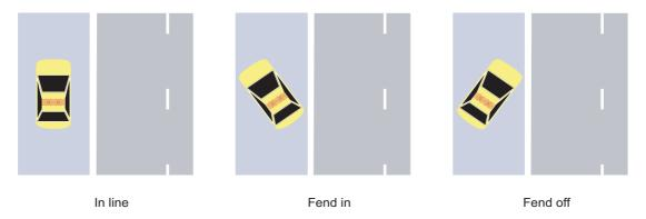
Figure 7.3 Positioning of vehicles
