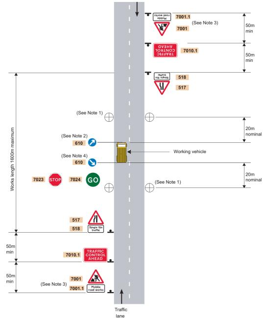
Plan SVW2: Single vehicle works on a single carriageway road – "STOP/GO"
