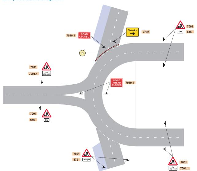
Plan MCC4: Mobile Carriageway Closure, closure of the upstream end of the access slip road – example of traffic management
