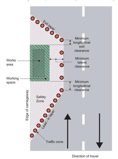
Figure 3.1 Safety zones – typical site layout
