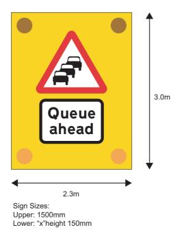
Figure 11.3 Vehicle-mounted queue warning sign
