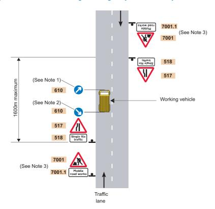
Plan SVW1: Single vehicle works on a single carriageway road, basic layout
