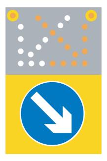
Figure 10.1 Light arrow system for block vehicles
