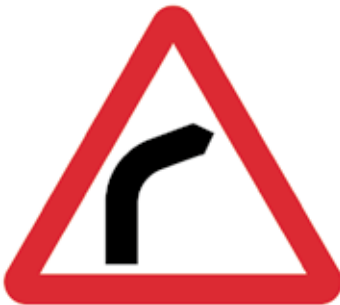
BEND TO THE RIGHT AHEAD Warning Sign
