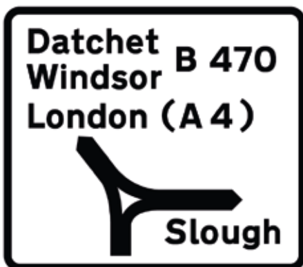
Advance Directional Informatory Sign
