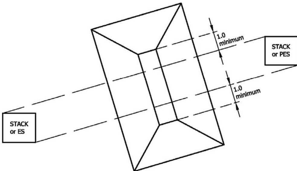
Figure 3 - Determination of Traverse Length
