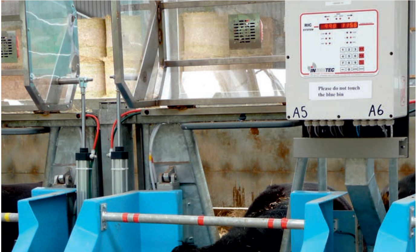
Above: SRUC 'GreenCow' facility for measuring greenhouse gas emissions from ruminants. Photographs supplied by Tony Waterhouse, SRUC
