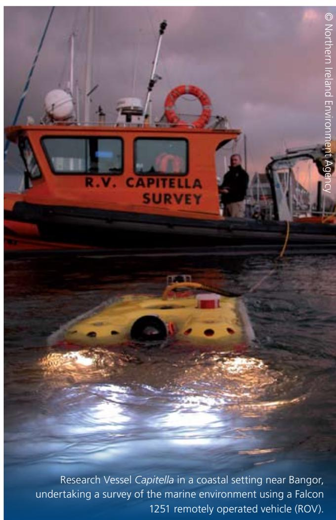
Research Vessel *Capitella* in a coastal setting near Bangor, undertaking a survey of the marine environment using a Falcon 1251 remotely operated vehicle (ROV).
