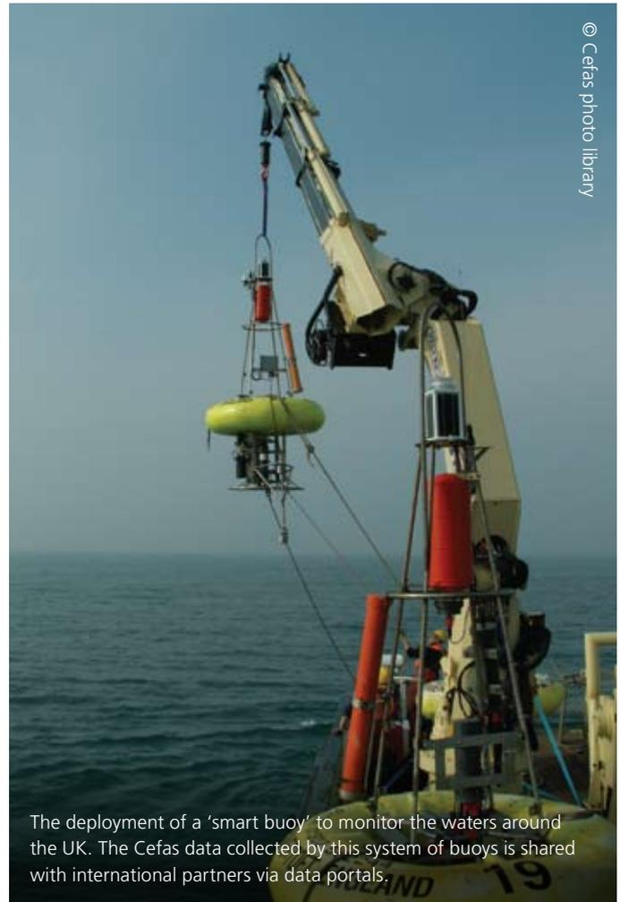
UK-designed 'smart buoys' provide rapid detection of environmental change in shelf sea waters with satellite-based data transmission.
