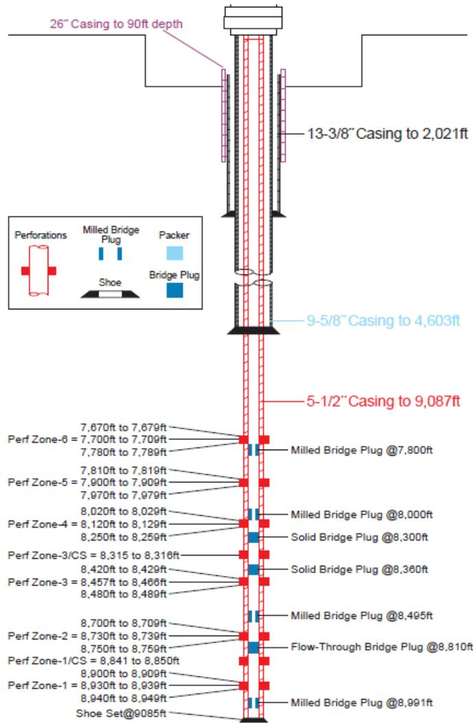
Figure 7: Cuadrilla completion schematic (Figure 11 Synthesis Report)
