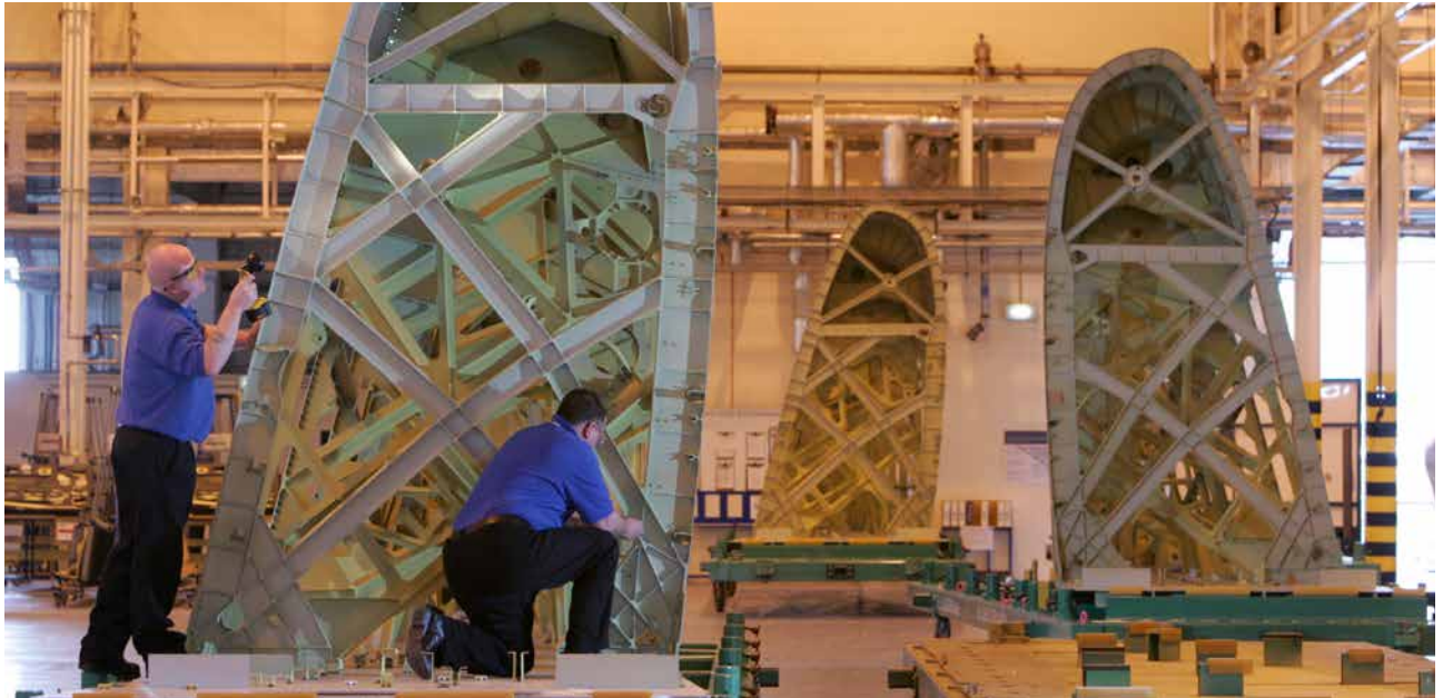
A380's inner outboard fixed leading edge wing assembly, produced at Spirit AeroSystems' site Prestwick, Scotland
