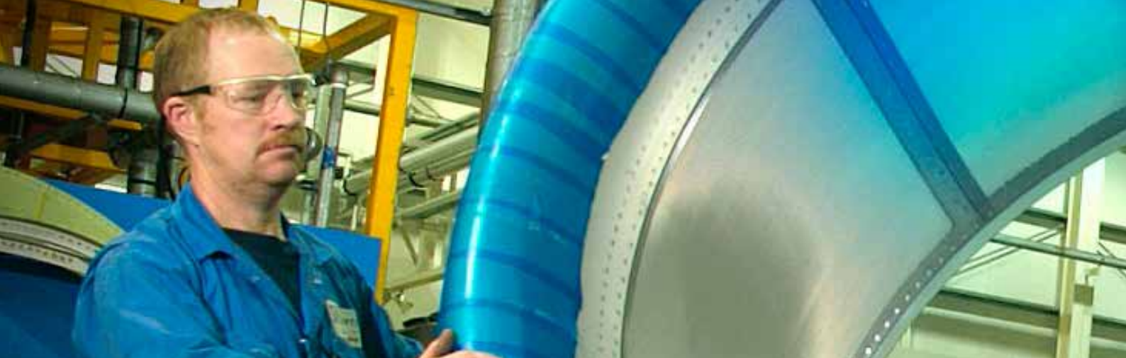
Inlet cowl on IAE V2500 engine, for the A320 aircraft, designed and manufactured by Bombardier, in Northern Ireland
