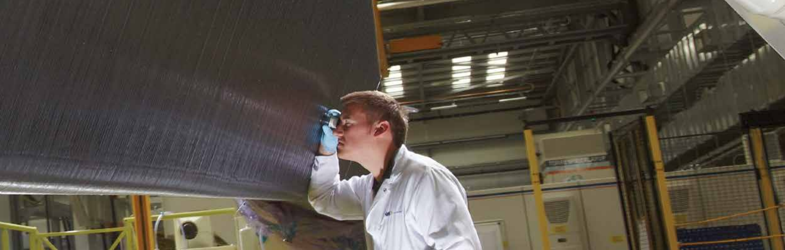
GKN, automated fibre placement on A350 rear wing spar, Filton, Bristol
