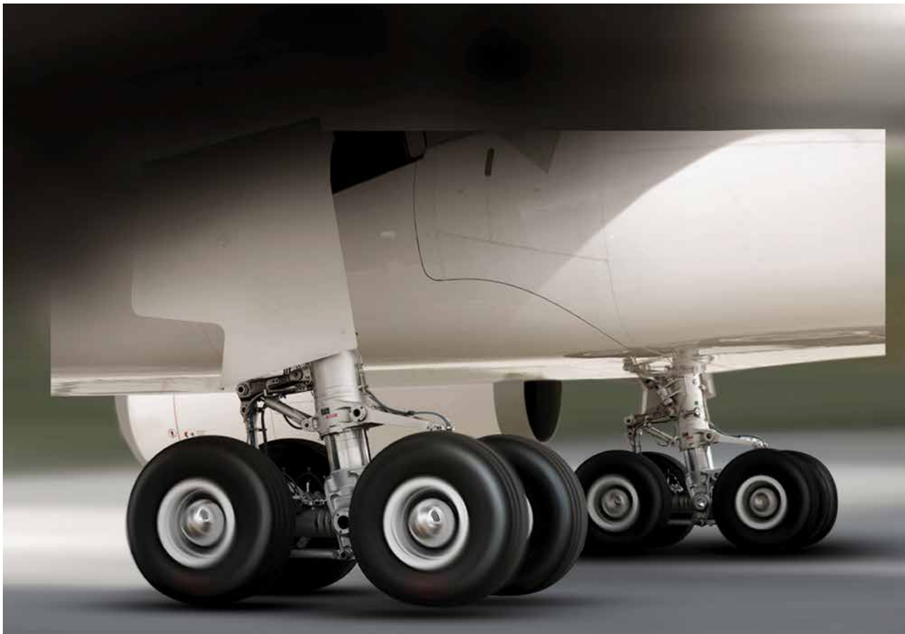
Airbus A330 main landing gear, designed and manufactured by Messier-Bugatti-Dowty, Gloucester Image © Messier-Bugatti-Dowty
