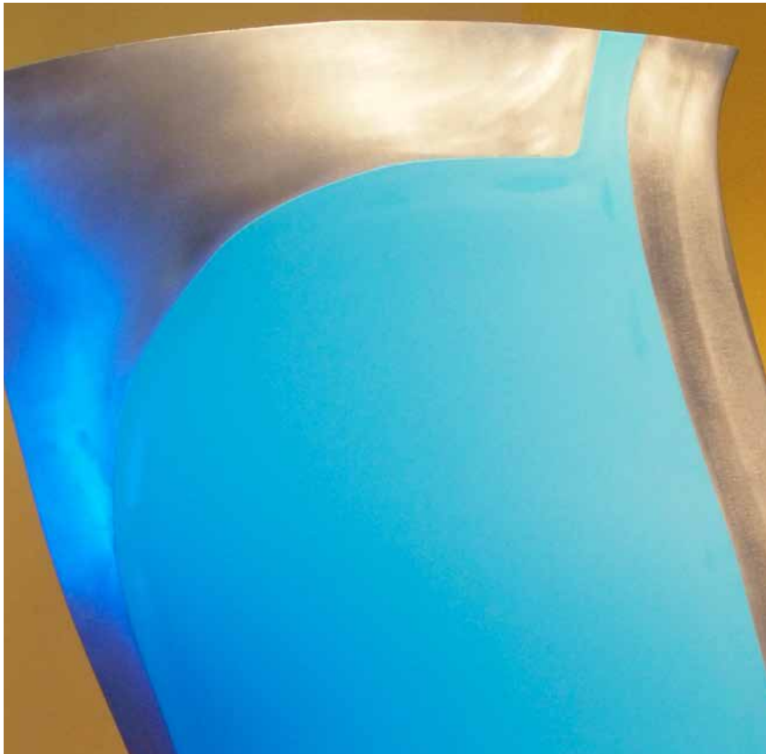
Composite fan blade, designed and developed in the UK
