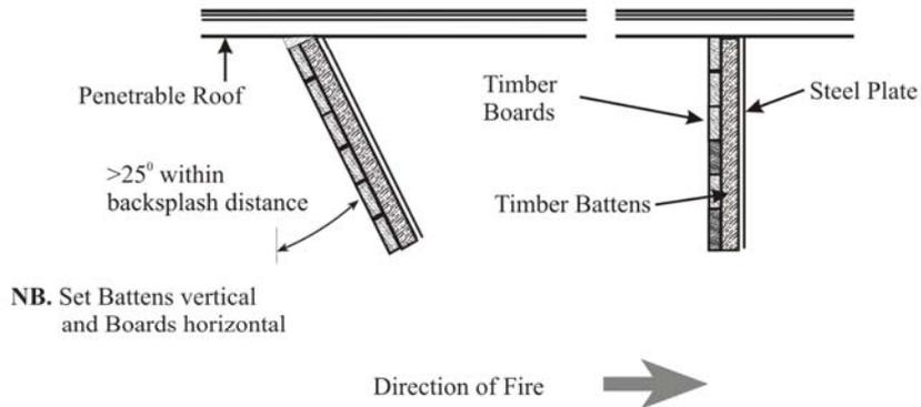
Figure 3-4. Baffle Construction
