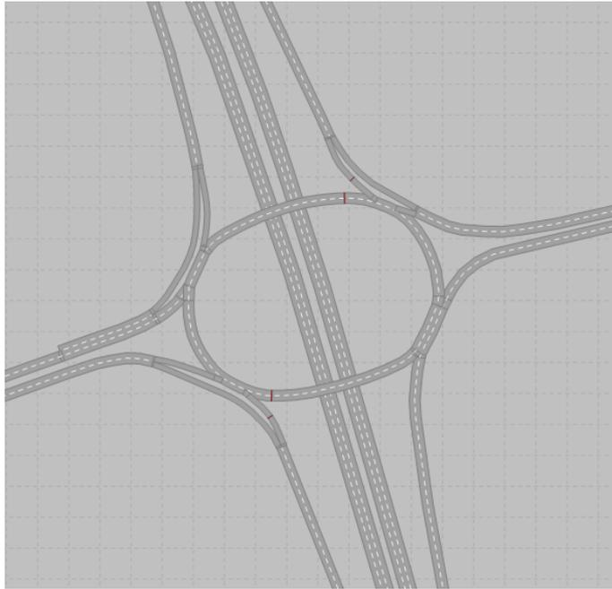
**Figure 8: Fully signalised grade separated roundabout**
