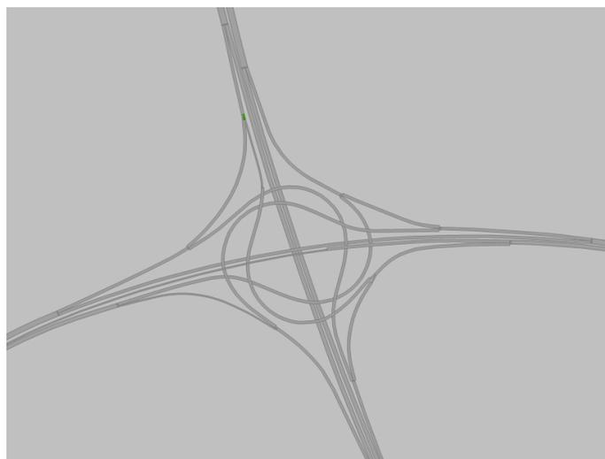
**Figure 7: Partially signalised grade separated roundabout**
