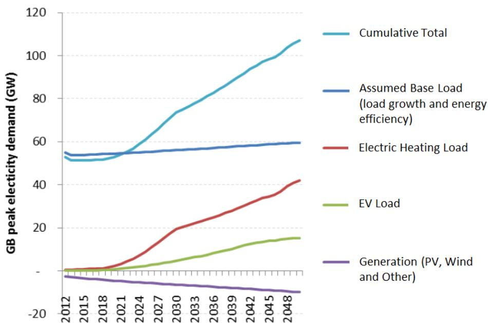
**Figure 2: Peak electricity demand for Scenario 1 showing the contribution of electric vehicle and electrified heating, together with the demand reduction effects of solar photovoltaics
