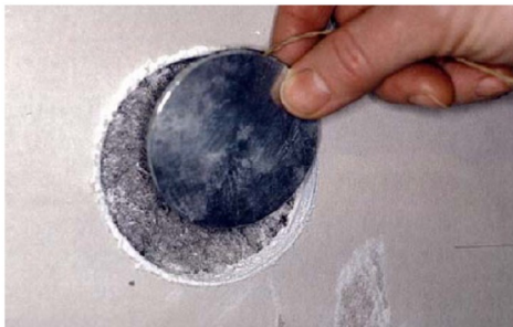
Figure 6: An embedded heat flux sensor being placed behind the interior gypsum board, from Figure 4 of the paper by Nicolajsen (2005).
