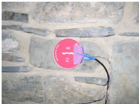
Figure 5: A surface-mounted heat flux sensor and temperature sensor (Rye 2010).
