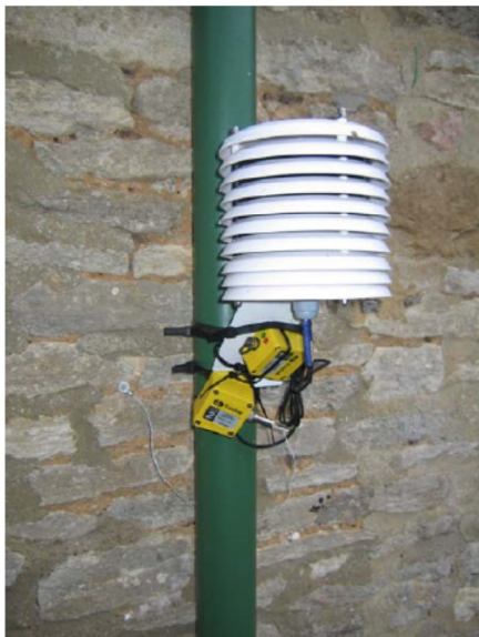
Figure 2: Examples of temperature sensors, sensing both the surface and the air temperature, Rye 2010.
